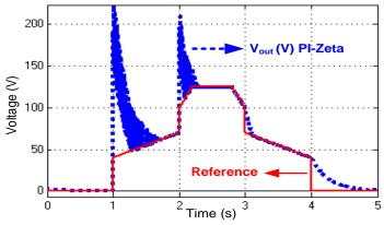
Figure 13. Change of the output voltage of the FLC controlled Zeta converter with the reference voltage.
