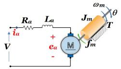
Figure 5. PMDC motor equivalent circuit.
