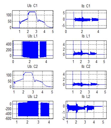
Figure 9. Zeta converter with PI controller components, current and voltage values change over time.
