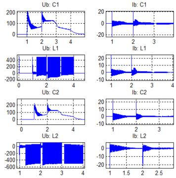
Figure 12. Zeta converter with FLC controller components, current and voltage values change over time.
