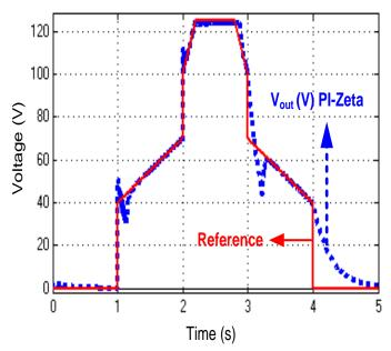
Figure 10. Change of the output voltage of the PI controlled Zeta converter with the reference voltage.
