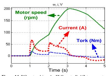
Figure 14. DC motor driven by FLC controlled Zeta converter.
